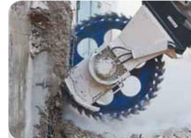
+ robust and exchangeable support brackets to modify cuttings depth
